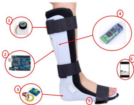
Fig.27. System Overview: 1) dc motor, 2) microprocessor, 3) piezoelectric sensor, 4) bluetooth module, 5) orthosis, 6) smart phone for mobile application
